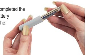
Use your remote control as you normally would. The remote and battery transmitter send the converted IR -> FR signals to the RF receiver. The RF receiver receives the RF signals and converts them back into IR.
